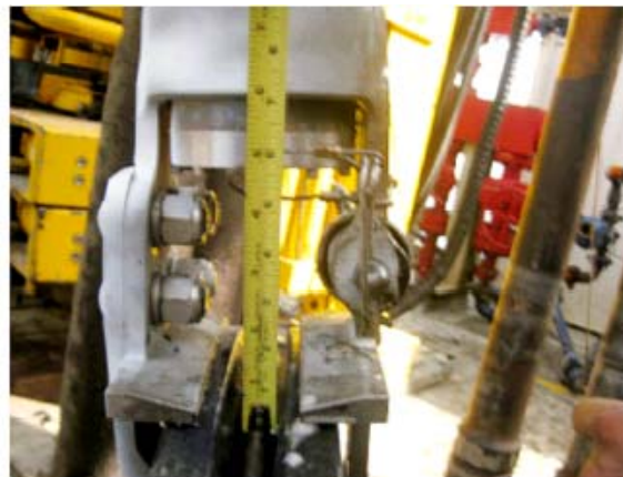
New sinker will not fit through top sheave
